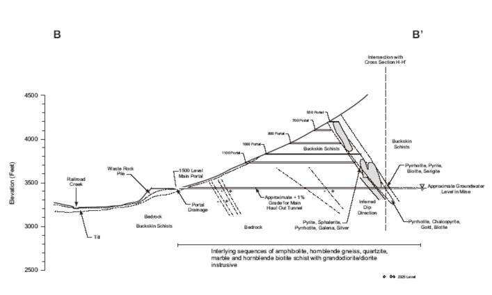
Note: This cross-section is generally perpendicular to ore body and parallel to 1500 level main tunnel.
